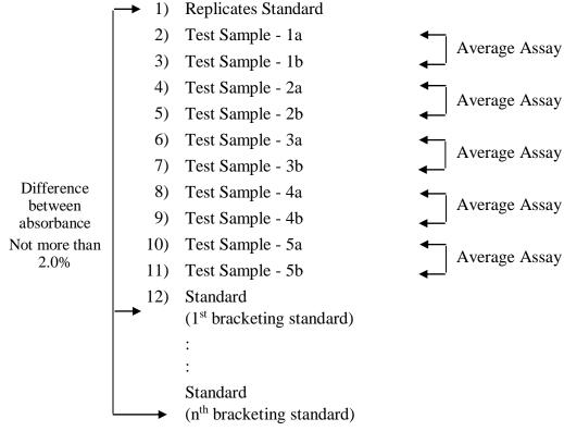
4.7 If the system is idle for 1 hour or more due to some minor problems that does not affect the system, then confirm the system is still suitable by injecting a bracketing standard before proceeding further.
