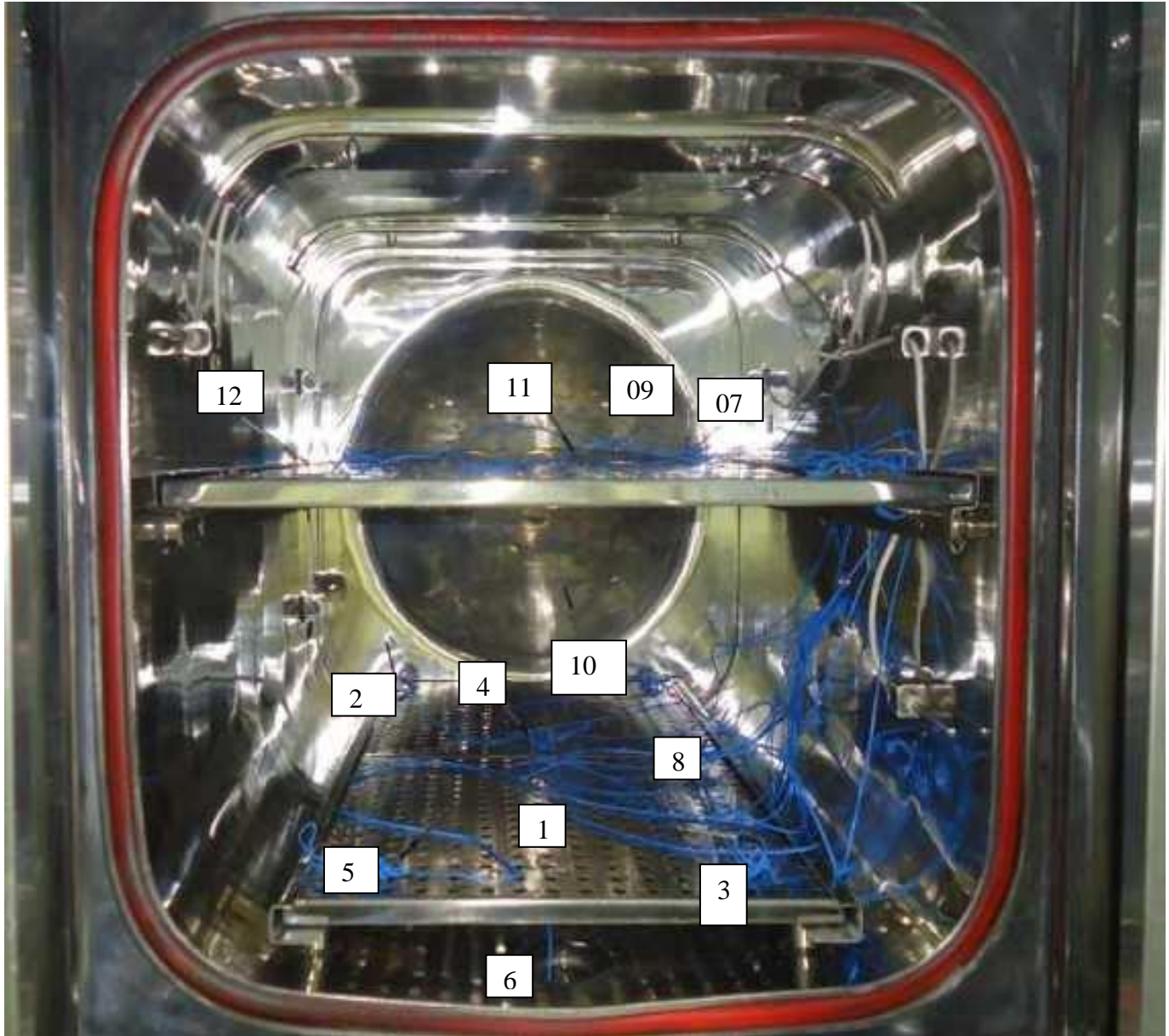
PHOTOGRAPH SHOWING LOCATION OF TEMPERATURE SENSORS IN EMPTY CHAMBER HEAT DISTRIBUTION STUDY INSIDE THE CHAMBER
