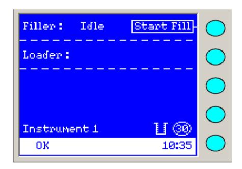
5.3.10 After completion of filling the blue light will start blinking near the filler section.
