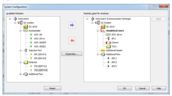
4.1.13.14 This window Configuration is only for Liquid Sample AOC 20i+s, SPL1 (liquid inject port) and TCD.
