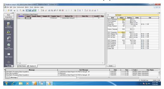
4.1.14.21.2 Click on file and open new batch file. Input Vial No., Sample name, Sample ID, Method file, Data file and Data description and then save batch file as per the required name.
