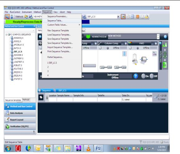
4.2.9.3 The sequence table by choosing the Injector source and completed the following entriese. Location,sample name,Method Name,Injection/ Location and sample type,injection Volume,vail Number.
