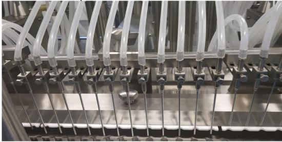
**6.2.3.5** Assemble Pre & Post Nitrogen needles manifold & connect the Nitrogen manifold outlet with needles by sterilized silicon tubing as below.
