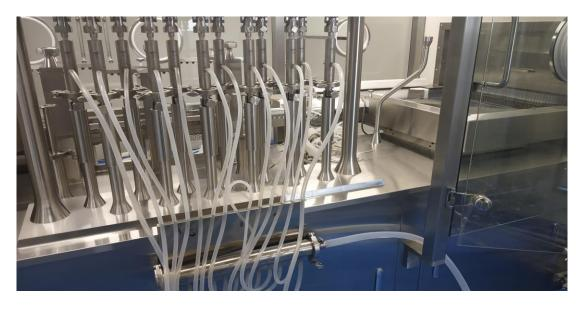
6.2.3.4 Connect the outlet of piston with filter needles shown as below.
