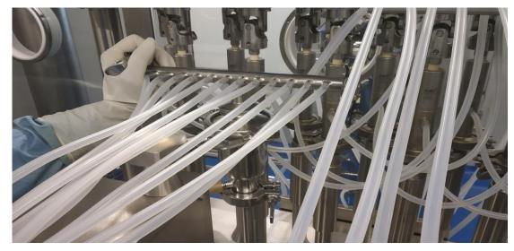
**6.2.3.3** Connect the inlet of piston with manifolds outlet by sterilized silicon tubing as below.
