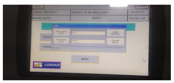
6.5 Now Press the "Menu" tab on the HMI screen & following screen shall display:
