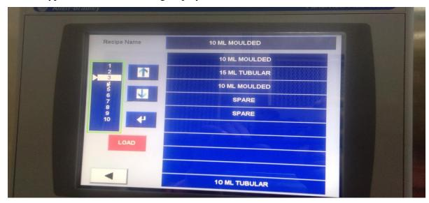
**6.8** Now following display shown in screen. Set temperature value and conveyor speed as per requirement.
