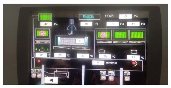
**6.11** Differential pressure of all zone such as Drying, Sterilizing, Cooling and Stabilizing Zone display as below:
