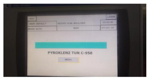
Now press "Login" tab on following screen display, press F2 for User Name and pass word for F3. Press login and enter.
