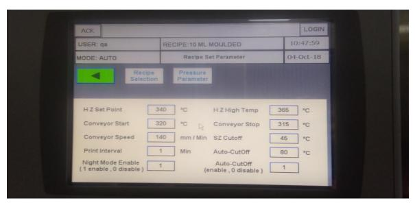
**6.9** Now the tunnel starts by pressing auto mode as shown on following display.
