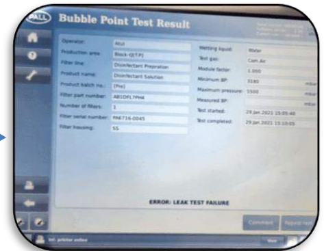
Error 2: Leak test failure
