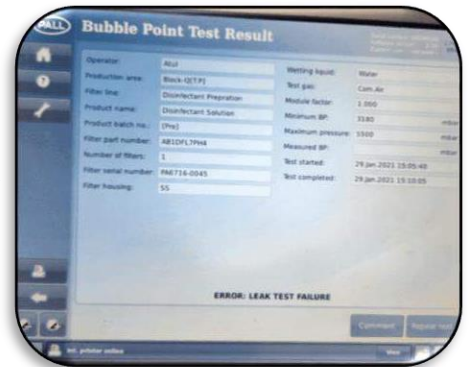
Error 2: Leak test failure
