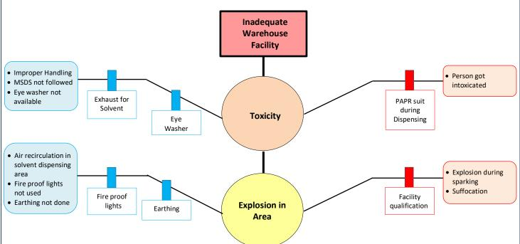
**SUMMARY OF THE BOW TIE ANALYSIS:** Bow Tie analysis for inadequate warehouse facility gives an overview of multiple plausible scenarios in a single picture. It provides a simple, visual explanation of a risk that would be much more difficult to explain.
