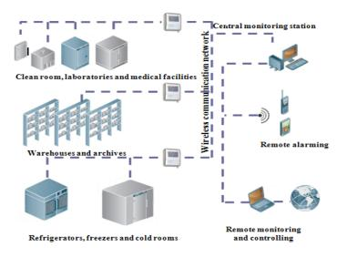
monitoring system combines efficient monitoring and controlling effective with alarming, simplified reporting records secure data & and storage.
