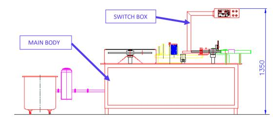
GA of Automatic External Ampoules Washing, Drying & Self Adhesive Labeling Machine:
