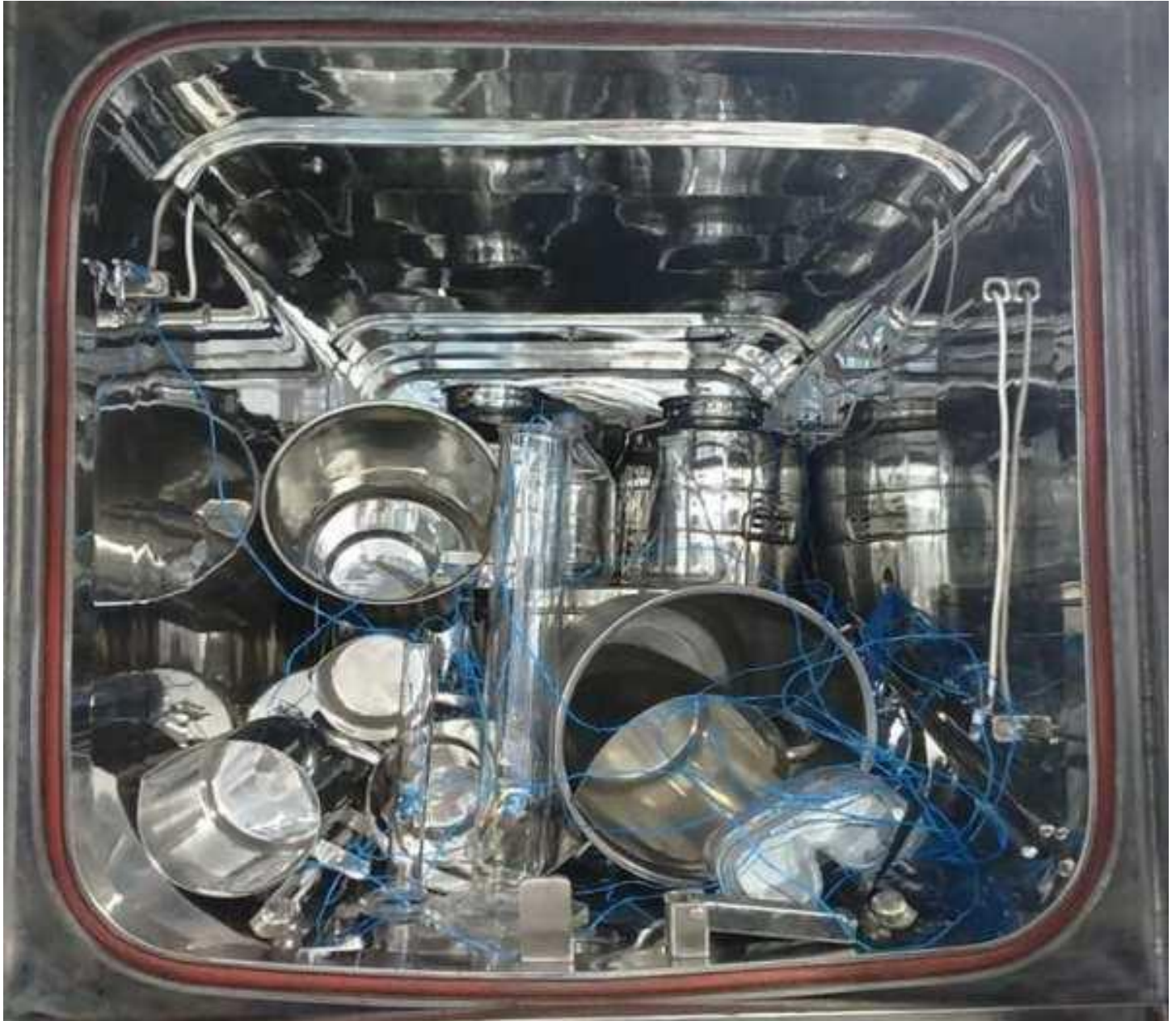
PHOTOGRAPH SHOWING LOCATION OF TEMPERATURE SENSORS IN FILTRATION ACCESSORY LOAD
