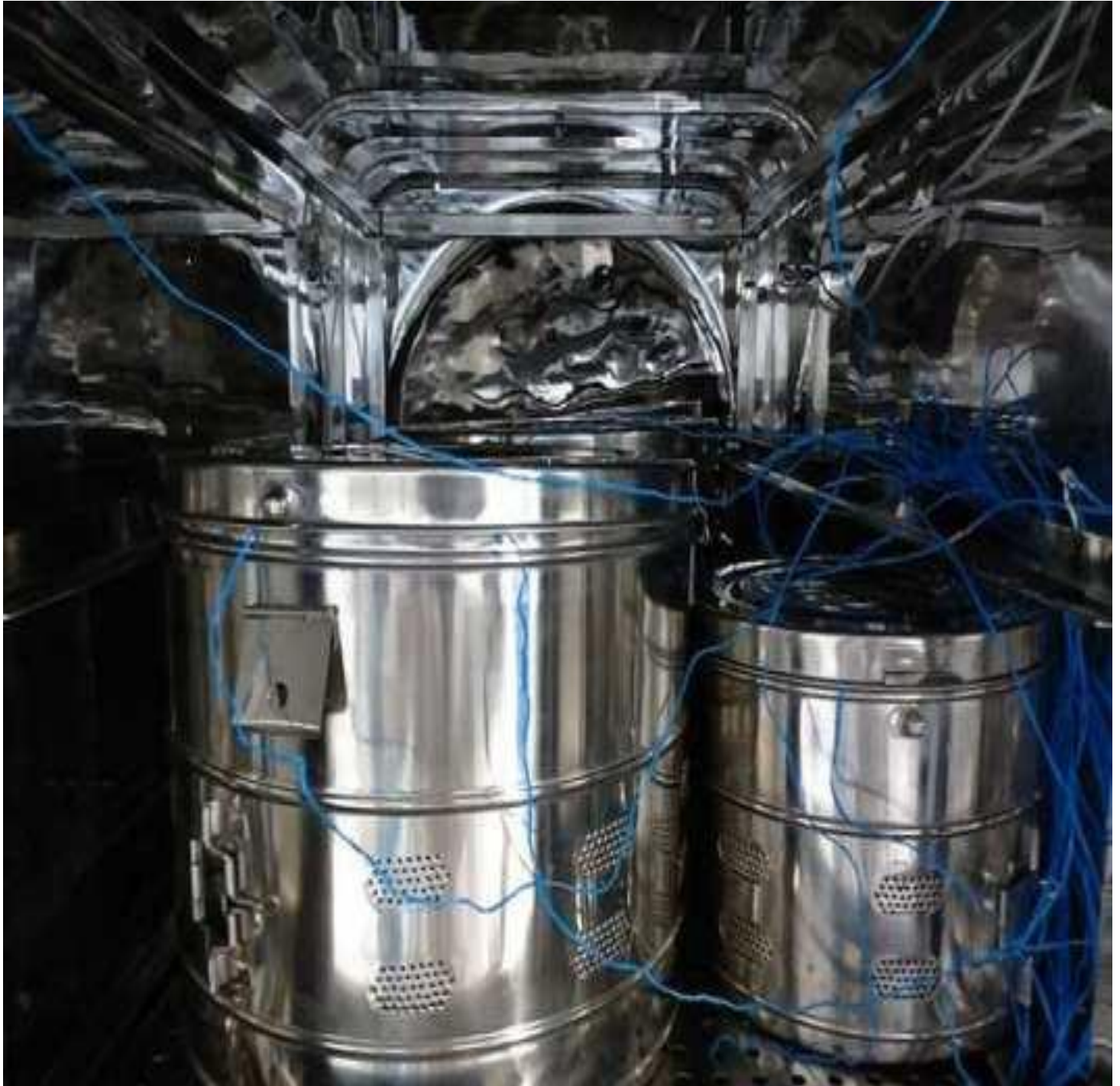
Photograph Showing Location Of Temperature Sensors In Empty Chamber Heat penetration Study in garment maximum load Inside The Chamber
