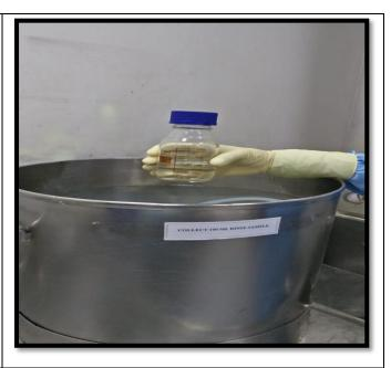
6. COLLECT APPROX 100ML RINSE SAMPLE (BY TILTING THE CONTAINER) AND PROCEED FOR DRYING OF CLEANED MACHINE PARTS USING FILTERED COMPERESSED AIR
