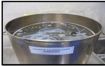
1. DIP UNCLEANED MACHINE PARTS IN PW FOR 15-20 MINS
