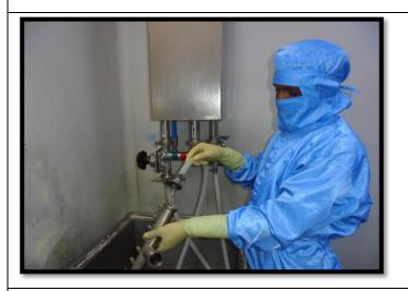
3. CLEAN ALL THE MACHINE PARTS THOROUGHLY WITH PW FOR 40-50 MIN
