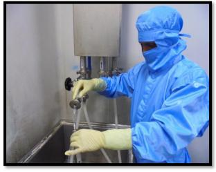
4. CLEAN ALL THE MACHINE PARTS THOROUGHLY WITH WFI FLUSH FOR 40-50 MINS
