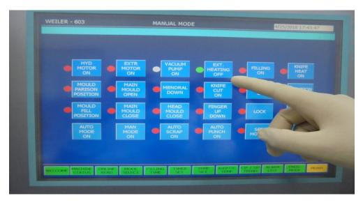
**6.3.7** Turn on the Knife heating from the Operator Panel.
