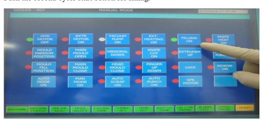
**6.3.25** Discard initially filled five cycle Bottles, Check for volume with 6<sup>th</sup> filled cycle & if volume is not within limit adjust the volume & proceed for further filling.
