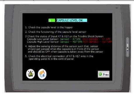
The following Alarm Info screen will be displayed incase of Powder level is low in the
