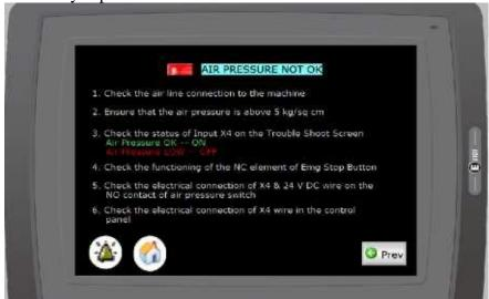
• The following Alarm Info screen will be displayed incase of Vacuum pump motor / blower motor / auger motor trip & Alarm Info key is pressed on Alarm screen.
