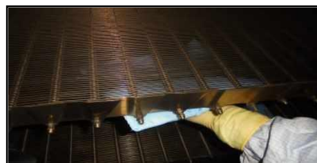
Conveyor cleaning (Lower side)
