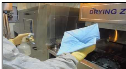
Drying zone cleaning (using 70% IPA)
