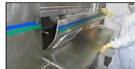
Remove side panel of cooling & stabilizing zone
