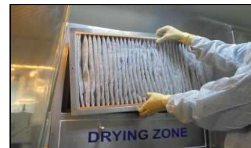
Remove Pre-filter for cleaning
