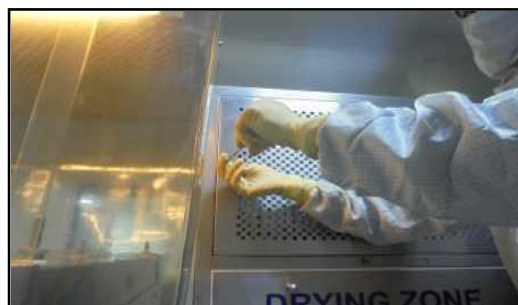
Open screw of Pre-filter grill
