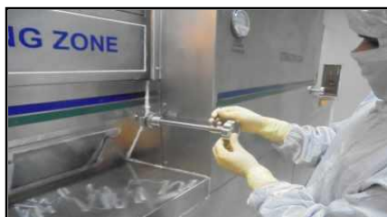
Open side panel of drying zone
