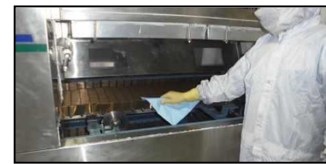
Cooling & Stabilizing zone cleaning (inside)
