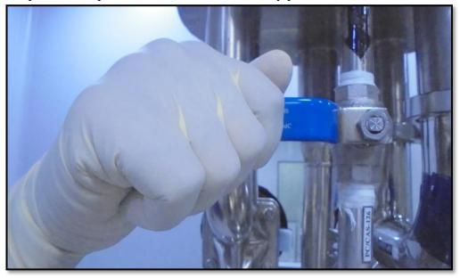
**6.8.5.3** Open the **purified & compressed air valve** located at bottom of tunnel.
