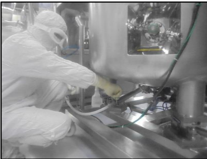
Connect the Silicon tubing with manifold to product line of filling vessel.
