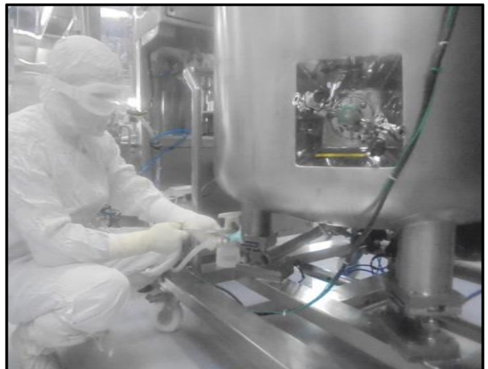
Connect the Silicon tubing with manifold to product line of filling vessel.
