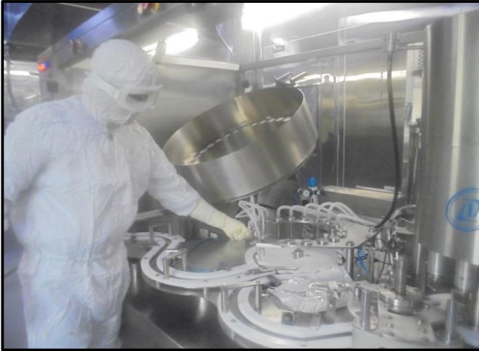
Connect the silicon tubing with manifold & purging needle
