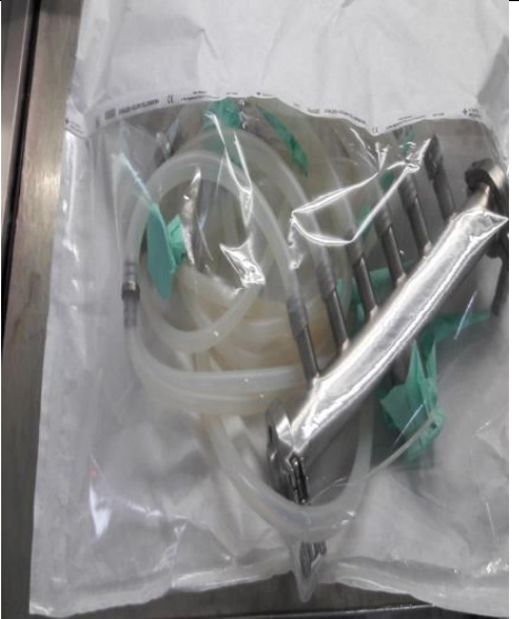
MANIFOLD WITH SS CONNECTOR SILICON TUBING AND FILLING NEEDLE
