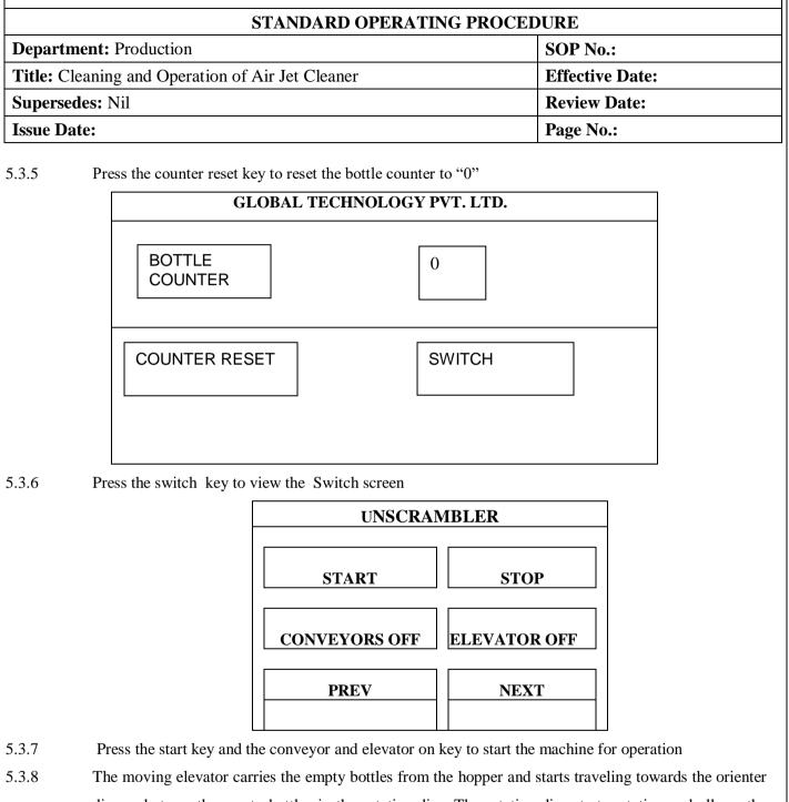
disc and stores the empty bottles in the rotating disc. The rotating disc starts rotating and allows the empty bottles to rotate from a line, where the rotating fan dos not allow the bottle jamming inside the rotating disc.
