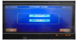
5.3.21 Select the "DY COMP." and it turn "ON" .Dynamic compensation is used to compensate the weight difference of the pack when it is in motion and in static condition.5.3.22 Select the "NEW DY. COMP." and then pass field bottle 20 times. The
