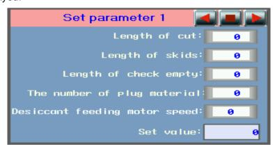
5.3.7 Press [Set Parameter] for setting the parameter. Before entering parameter set interface, operator has to input correct password.
