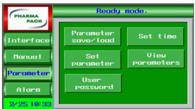
5.3.5 Parameter: By pressing [Parameter] icon in touch screen at Operation Interface following will be displayed.
