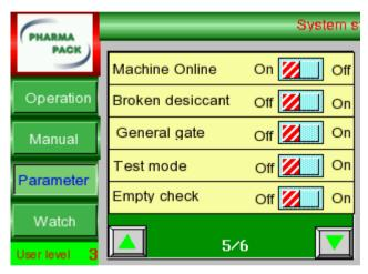
Broken desiccant: when this button is OFF, broken desiccant detect function is off. when this button is ON, broken desiccant will be detected and rejected.
