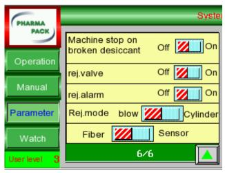
Machine stop on broken desiccant: when this button is OFF, broken desiccant detect function is off. when this button is ON, broken desiccant will be detected and rejected.
