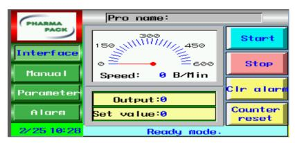
5.3.3 Click button [Interface], [Function], [Alarm] to switch to these different interfaces.
