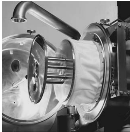
FIGURE 7.17 Open bowl of HF inverting filter centrifuge. (Image courtesy of HEINKEL AG.)
