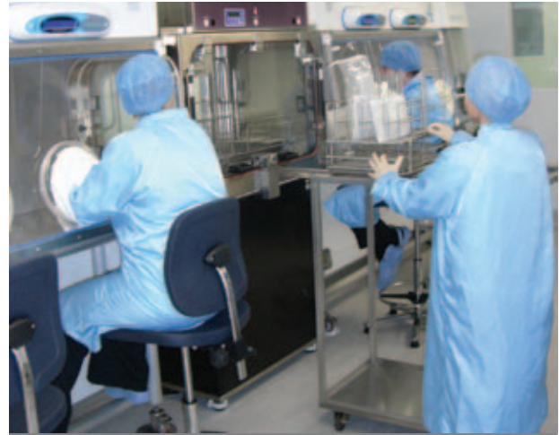
Cleanroom barrier isolator. Image courtesy of Bioquell UK Ltd
