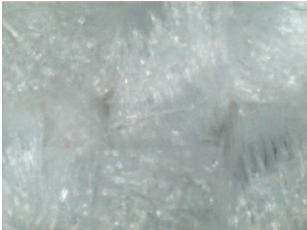
Photomicrograph of polycotton fabric
