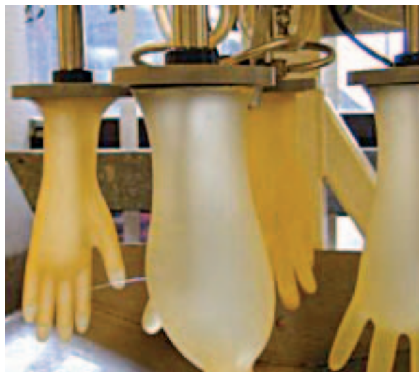
Automated glove leak testing machine
