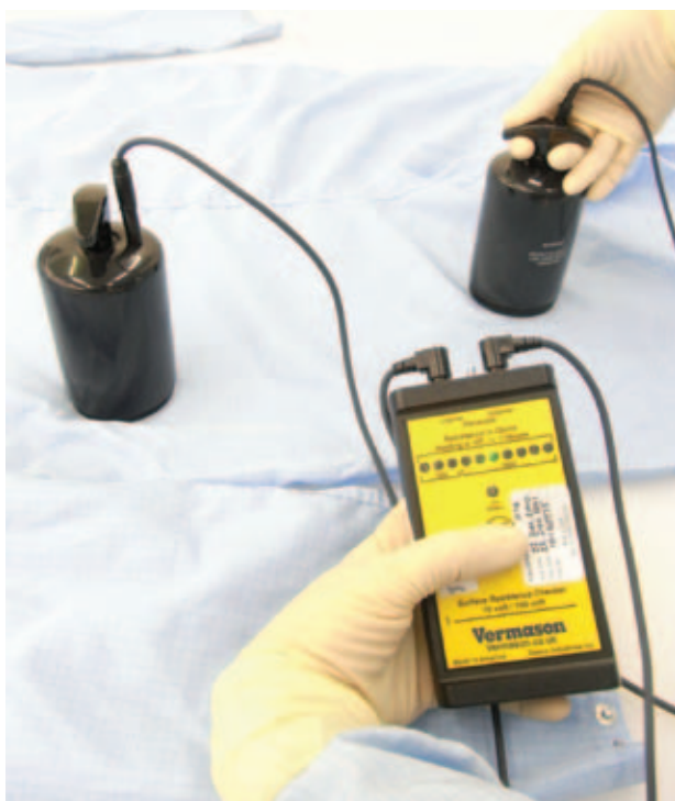
ESD testing of cleanroom clothing
