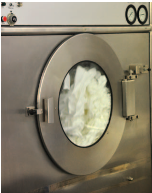
Cleanroom tumble dryer in operation
