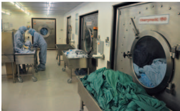
Cleanroom clothing being processed in a decontamination plant
