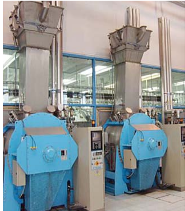
Barrier washer extractor machines incorporated into the cleanroom wall to act as a pass-through barrier into the processing cleanroom
