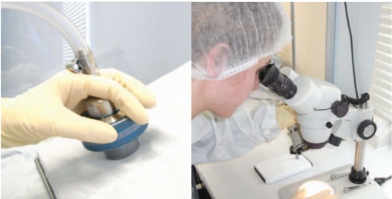
ASTM F51/00 particulate test, removal of particles and microscopic evaluation
