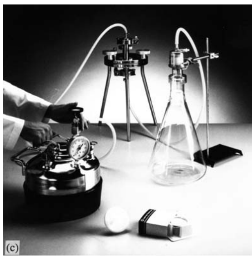
Figure 3.28. Photographic representation of a range of filter types and their stainless steel housing. Most filters used on an industrial scale are of a pleated cartridge design which facilitates housing of maximum filter area within a compact space (a). These are generally housed in stainless steel housing units (b). Some process operations, however, still make use of flat (disc) filters, which are housed in a tripod-based stainless steel housing (c). Photos courtesy of Pall Life Sciences, Ireland
