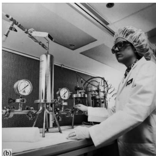
Figure 3.28. Photographic representation of a range of filter types and their stainless steel housing. Most filters used on an industrial scale are of a pleated cartridge design which facilitates housing of maximum filter area within a compact space (a). These are generally housed in stainless steel housing units (b). Some process operations, however, still make use of flat (disc) filters, which are housed in a tripod-based stainless steel housing (c). Photos courtesy of Pall Life Sciences, Ireland
