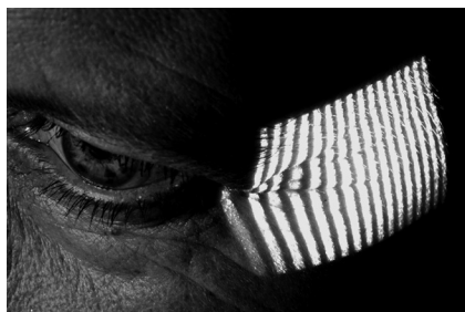
FIGURE 20.1 Distortion of the regular sinusoidal fringe pattern by the irregular surface of the skin. Presentation of crow's feet (wrinkles that appear around the eye, classically starting at the outer corner of the eye).
