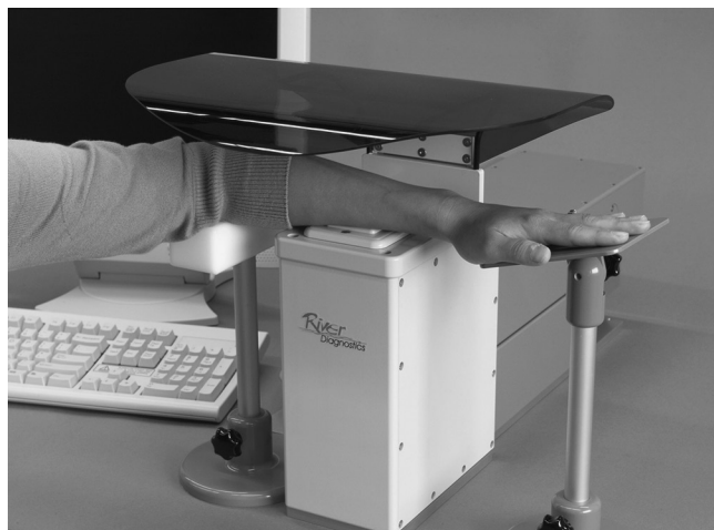
FIGURE 10.1 The RiverD International Model 3510 Skin Composition Analyzer is the first Raman instrument optimized for in vivo analysis of skin.
