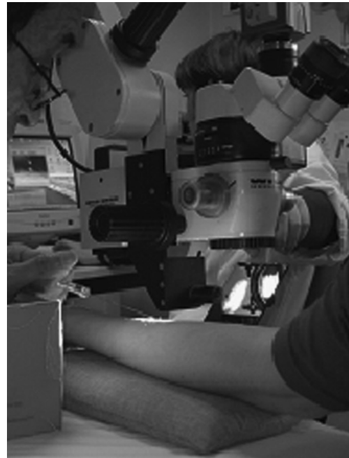
FIGURE 30.4 Contact angle visualization and measurement: measurements are based on the use of a mirror directed 45^\circ to the skin; “profile drop method.”
