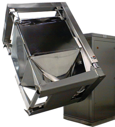
Figure 8.6: Typical IBC Blending Unit
