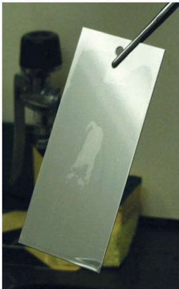
Figure 5.8: Image of a Stainless Steel Coupon used for a Laboratory Cleaning Evaluation Used with permission from STERIS, www.steris.com .
