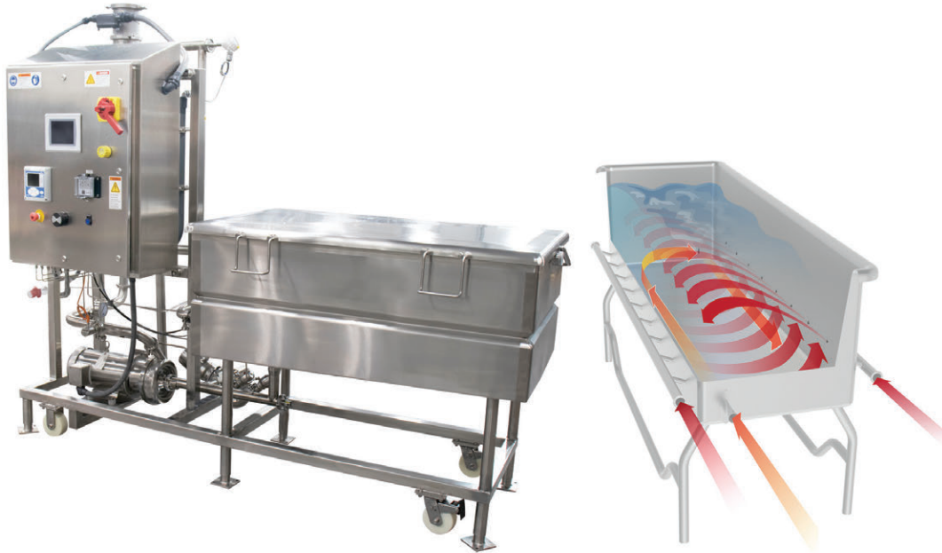
Figure 5.6: Example of Clean Out Of Place (COP) System on Left and Model of Combined Push-Pull and Rotational Flow through Rectangular Tank on Right
