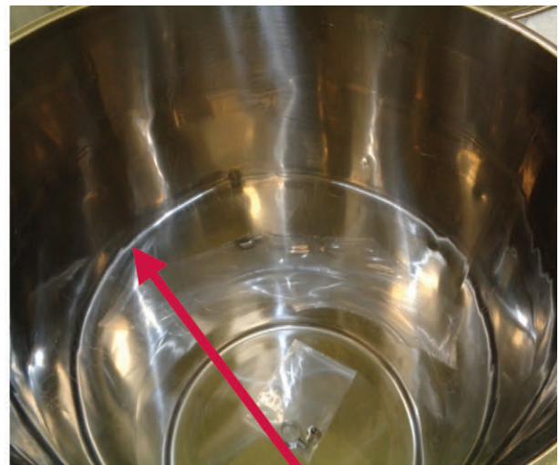
Side of Tank at Fill Line
