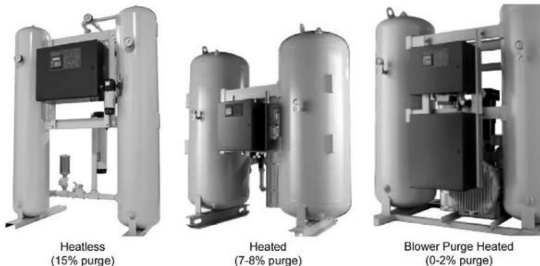
Figure 4.5: Types of Regenerative Desiccant Type Air Dryer
