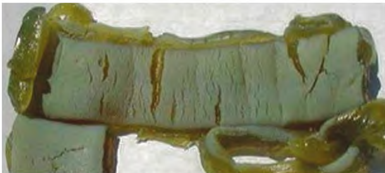
Figure 8.3: Example of Urethane Gel Developing Toughening and Cracking on the Surface
