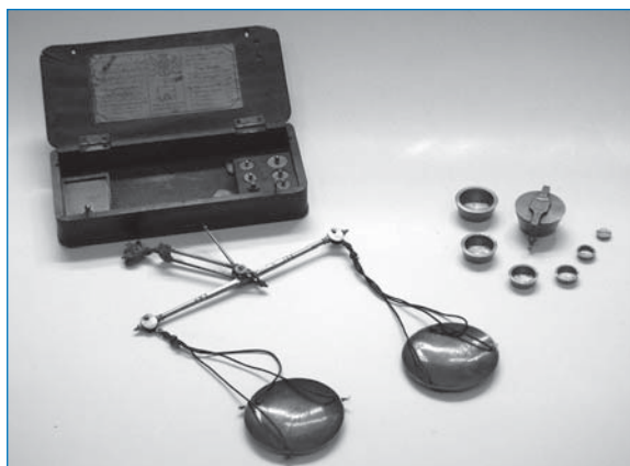
Figure 2.9 A pair of hand-scales with box-end beam, silver pans and brass apothecary weights, made by Young and Son, 1814–1815.
