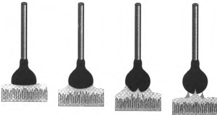
Figure 4 Schematic diagram showing the progression of bioadhesive fracture.
