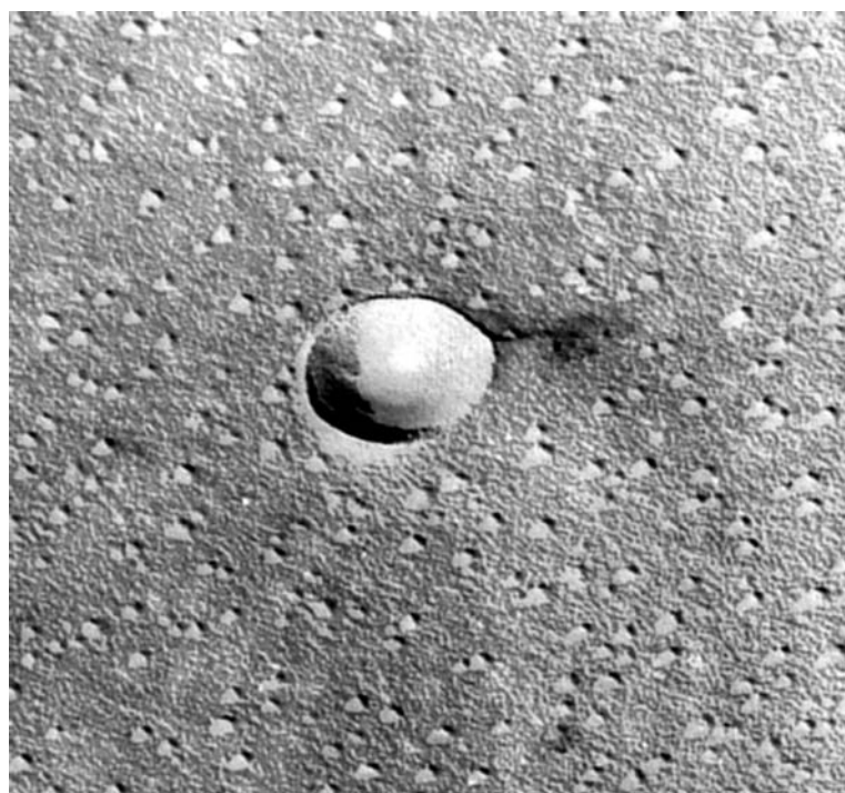
Figure 7 TEM photomicrograph of amphiphilic \beta -cyclodextrin nanocapsules after freeze-fracture ( \times 31,500 ). Abbreviation: TEM, transmission electron microscopy. Source: From Ref. 41.
