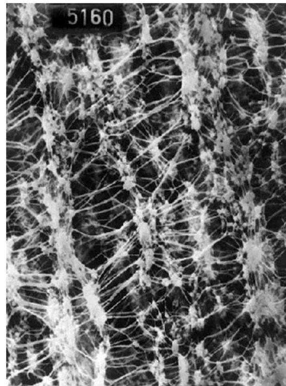
Fig. 5 PTFE membrane structure. (Courtesy of Sartorius AG.)
