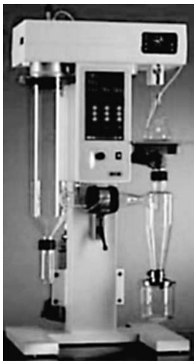
Fig. 7 Buchi/Brinkmann Lab Scale Spray-Dryer. A stock solution or suspension is pumped from the beaker through a nozzle which sits above the large glass particle formation vessel on the left-hand side. The nozzle atomizes the feedstock at temperatures ranging from ambient to 250°C into the particle formation vessel, using air or an inert gas such as nitrogen to dry and move particles into the cyclone and collection chamber on the right-hand side. Product temperature is monitored by a temperature probe mounted between the particle formation vessel and the cyclone. Solvent or water are exhausted through a fine particle filter bag in series with the cyclone, which also collects fines.
