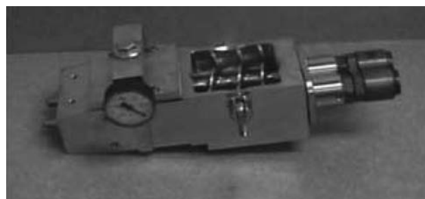
Fig. 6 Twin horizontal feed screw system with vacuum deaeration. (Courtesy of Alexanderwerk Inc.)
