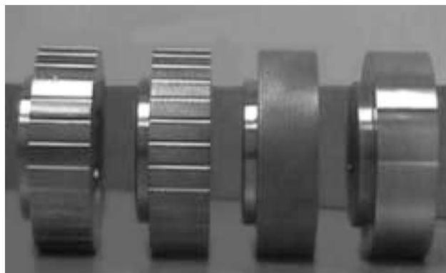
Fig. 8 Roll configuration designs. (Courtesy of Alexanderwerk Inc.)
