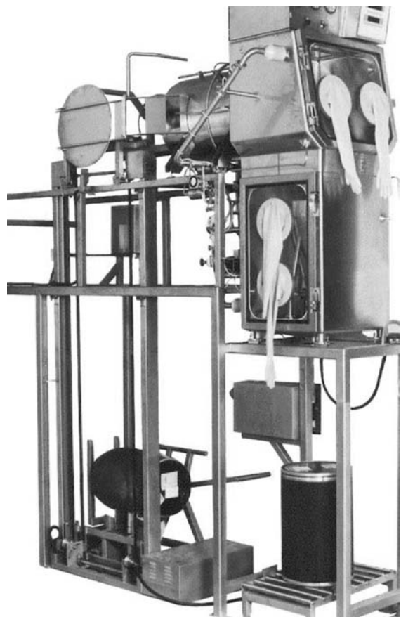
Fig. 2 Potent drug-dispensing isolator. (Photograph courtesy of TPC Microflow Ltd.)
