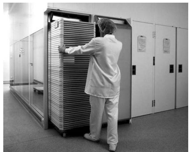
Fig. 9 Tray drying of Softgels in controlled drying tunnels.
