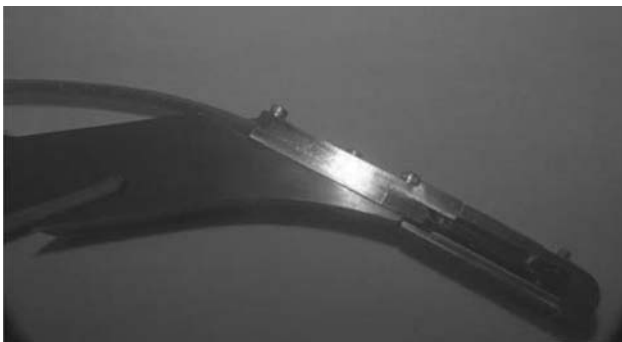
Fig. 6 Instrumented take-off bar.
