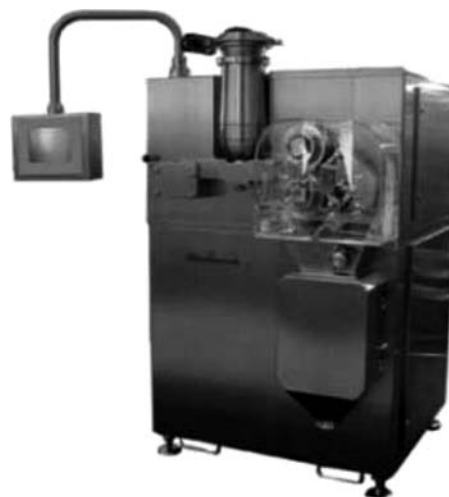
Fig. 18 Computer controlled roller compactor with horizontal feed screws, vacuum deaeration, and cantilevered rolls. (Courtesy of Alexanderwerk Inc.)
