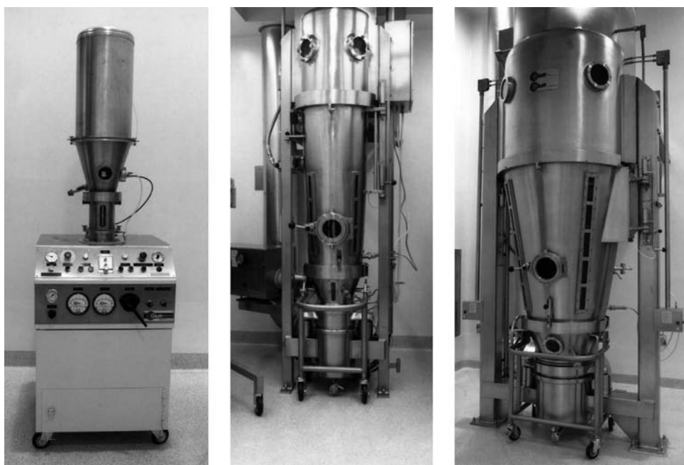
Fig. 1 Fluid-bed granulator driers of 1, 5, and 50 kg capacity, which provide flexible clinical supplies manufacturing capacity and can be used to understand critical process variables and scaling parameters.
