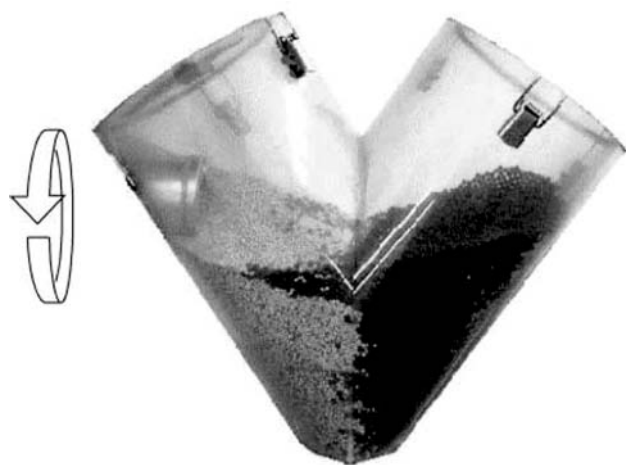
Fig. 1 “Left-right” segregated state, here in a transparent V-blender, between larger (dark) and smaller (light) grains. This state occurs spontaneously at high fill levels and fast tumbling speeds in many tumbler designs.
