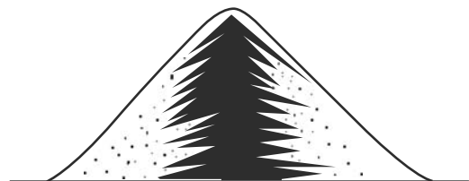
Fig. 7 Segregation in powder heaps. Finer particles are illustrated in black and coarser particles are in white. (Reprinted from Ref. [5] by courtesy of Marcel Dekker, Inc.)
