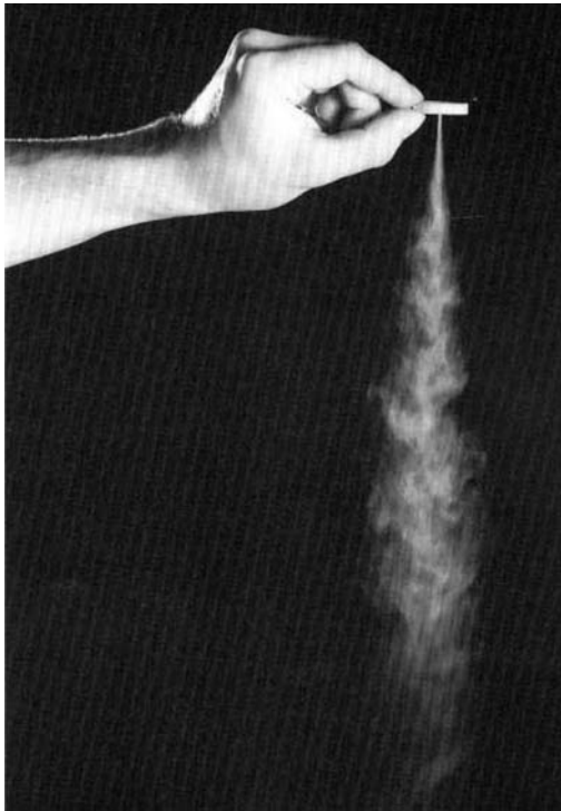
Fig. 4 Inhalation droplet spray plume produced by Touch-Spray device. (Reproduced courtesy of The Technology Partnership plc, UK.)
