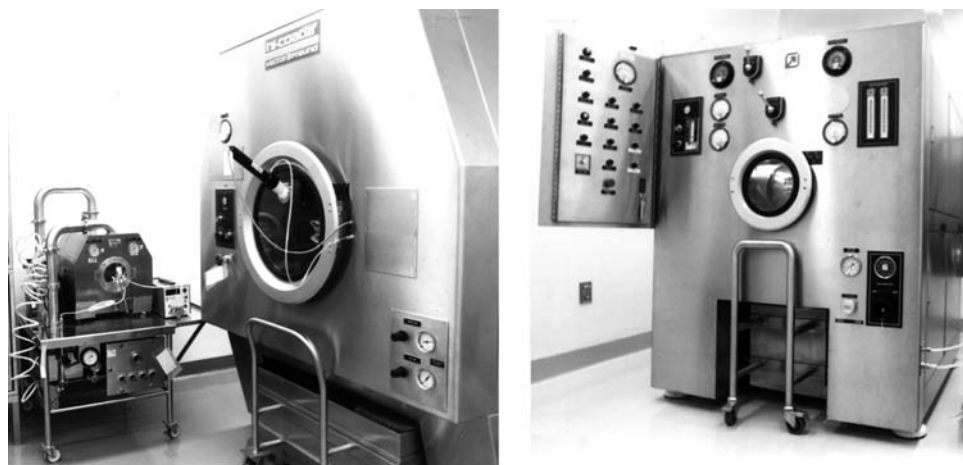
Fig. 2 Coating pans of 1, 15, and 150 kg capacity.
