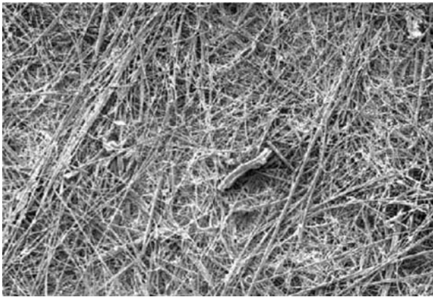
Fig. 3 SEM of the random fiber matrix of a depth filter. (Courtesy of Sartorius AG.)
