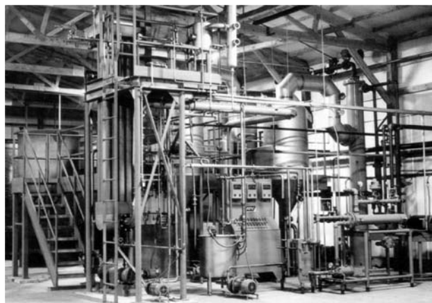
Fig. 2 Two-effect rising/falling film plate evaporator. (Courtesy of APV Crepaco, Inc., APV Americas, Rosemont, IL—An Invensys Company.)
