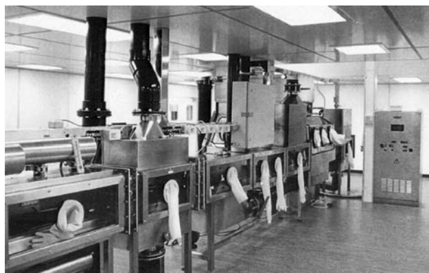
Fig. 5 A specialized network of isolators used for large-scale industrial syringe filling; process flow is from left to right. (Photograph courtesy of Medeva Ltd.)
