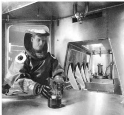
Fig. 3 Specialized isolator for potent drug processing and handling. (Photograph courtesy of TPC Microflow Ltd.)
