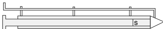
Fig. 2 The unit-dose compacting sample thief. The sample is collected in the “S” section and the outer rod rotates to open and close the thief. (Reprinted from Ref. [5] by courtesy of Marcel Dekker, Inc.)
