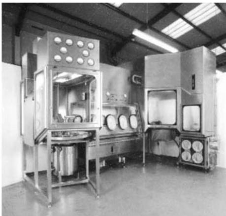
Fig. 3 Specialized isolator for potent drug processing and handling. (Photograph courtesy of TPC Microflow Ltd.)
