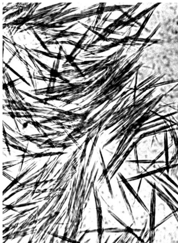
Fig. 2 Optical micrograph of Merck pharmaceutical crystals with good filterability (200 \times ).
