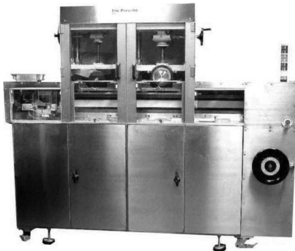
Fig. 21 Tablet press replicator: The Presster™.
