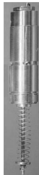
Fig. 2 Linear variable differential transformer (LVDT).
