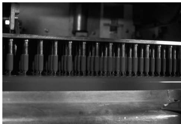
Fig. 2 Dip pan, capsule shell formation. (Reprinted with permission from Qualicaps Europe, S.A.)
