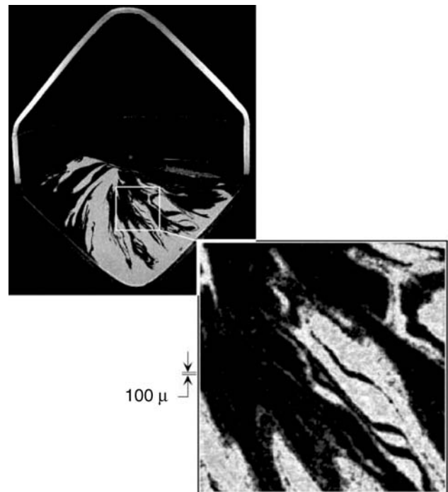
Fig. 23 High-resolution data are obtainable by solidifying and slicing an entire blend, here of identical but colored \sim 90\text{-}\mu\text{m} grains in a double-cone blender.
