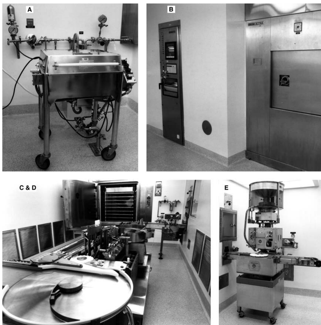
Fig. 1 Sterile dosage form processing equipment useful for clinical supply manufacture in the pilot plant. (A) Vial and ampule washer (Metromatic, Oyster Bay, NY). (B) Steam sterilizer (Amsco Finn-Aqua, Apex, NC). (C) Vial filler (TL Systems Corp., Minneapolis). (D) Lyophilizer (Edwards High Vacuum International, Tonawanda, NY). (E) Vial capper (The West Co., Phoenixville, PA).
