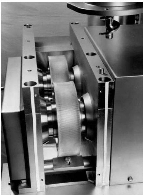
Fig. 21 Fixed rolls on two bearing blocks, rolls are concave. (Courtesy of Bepex-Hosokawa Co.)
