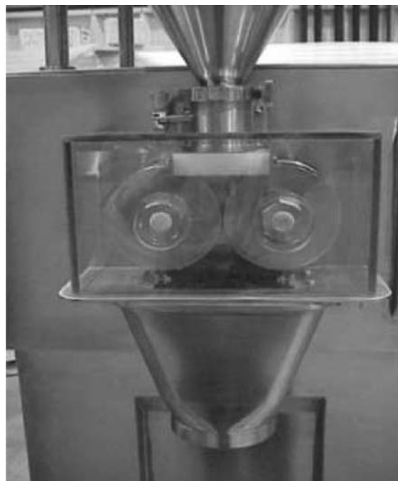
Fig. 22 Cantilevered compactor with one fixed and floating rolls, no vacuum deaeration, sizing device not attached. (Courtesy of Vector Co.)
