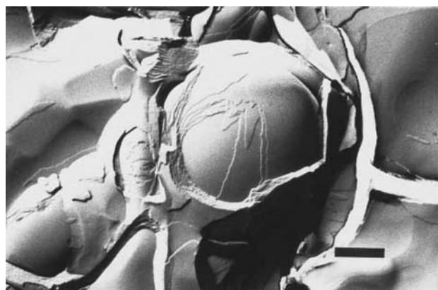
Fig. 13 Transmission electron micrograph of a freeze fractured w/o cream. The aqueous phase is dispersed as droplets within the continuous lipophilic phase and the interface consists of multiple bilayers of hydrated surfactant molecules; bar 500 nm. (From Ref. [41] )
