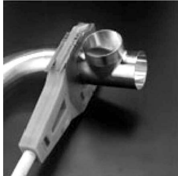
Fig. 4 Automatic orbital welder in the process of joining two long tangent stainless steel fittings.
