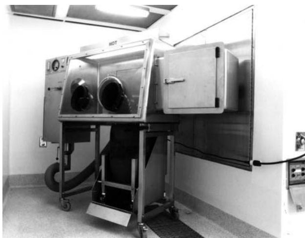
Fig. 9 Containment unit built for dispensing small quantities of highly active compounds.
