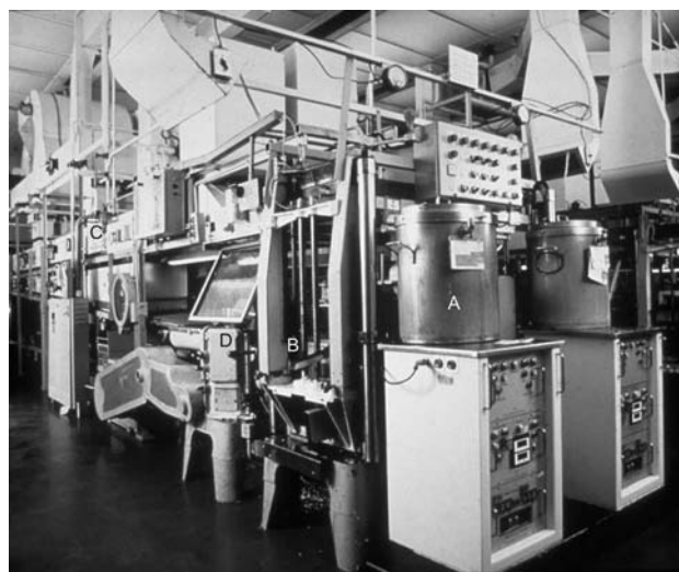
Fig. 1 A capsule manufacturing machine: (A) gelatin solution storage tank; (B) dip pan; (C) drying kilns; and (D) Automatic section. (Reprinted with permission from Eli Lilly & Co. Ltd.)
