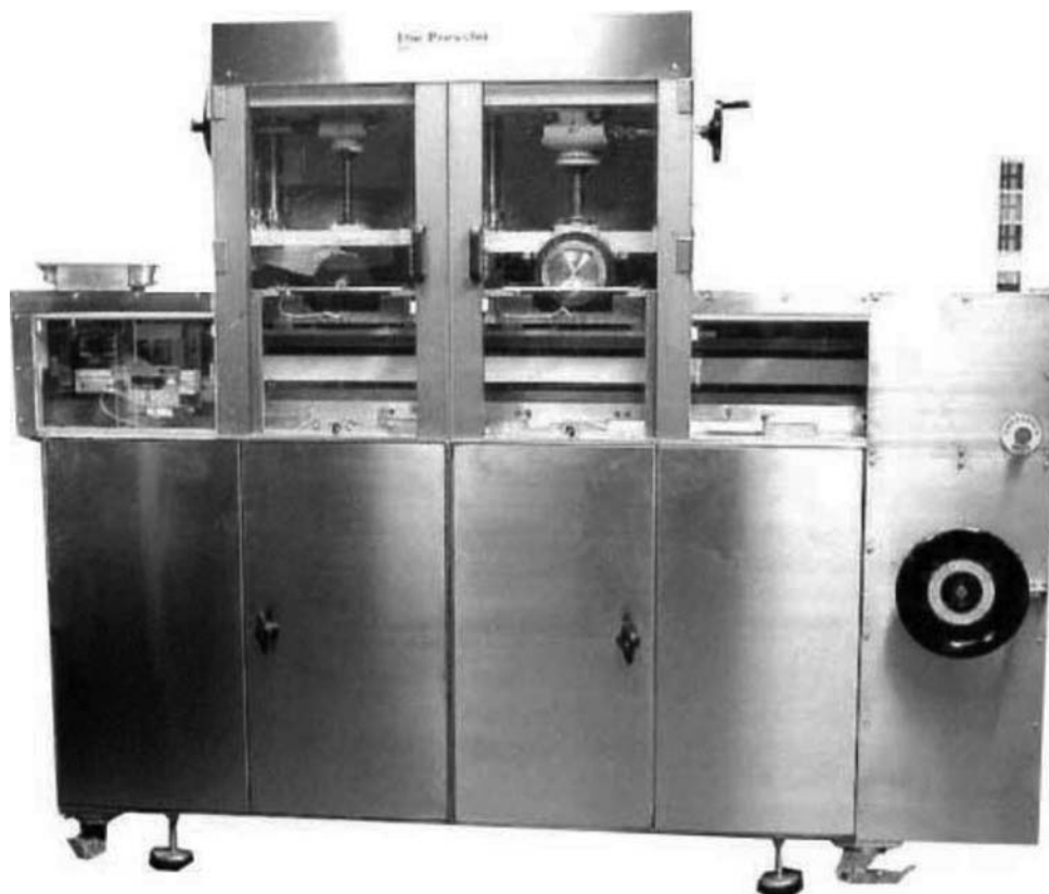
Fig. 21 Tablet press replicator: The Presster™.
