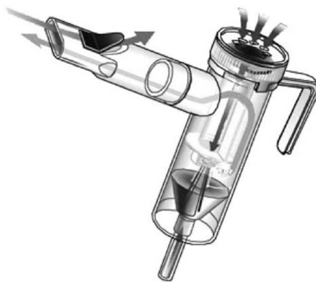
Fig. 6 The diagram of the Pari LC Plus jet nebulizer. (Courtesy of Pari GmbH.)
