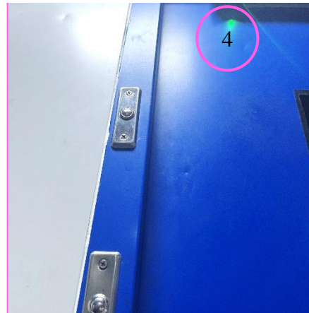
Figure 2: In case of door opening, shows Red indicator Figure 3: Green indicator (Encircled), in case of door closed (Encircled) completely
