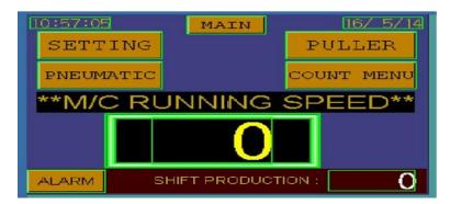
5.5.10 Now select the parameters in setting menu and put value as desired for setting of machine and go through the NEXT button on PLC to select other parameters.
