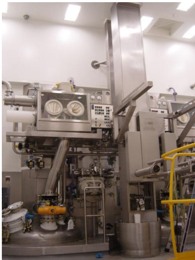
Charging a reactor using a lifting column
