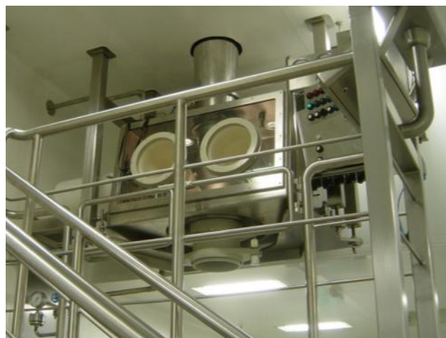
Discharging a dryer into FIBCs
