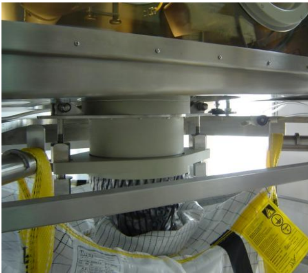
Filling a FIBC connected to an isolator
