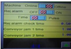
NOTE: "PARAMETER" has three pages displayed as 1/4, 2/4, 3/4, 4/4. we can switch into different pages by pressing  $\triangle$   $\nabla$ . Each of the parameter displayed (numeric value) can be edited. Press the number and key pad will be displayed which will help in entering the value, then press "ENTER".
