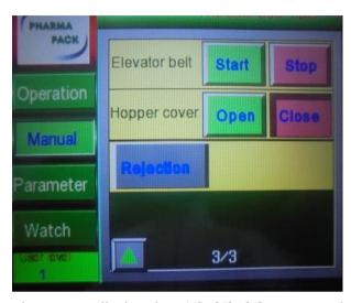
**Note:** - "MANNUAL" has three pages displayed as 1/3, 2/3, 3/3 we can switch into different pages for different parameters by pressing  $\square$   $\square$ . Each of the parameter displayed can be "START" and "STOP" by pressing the key.
