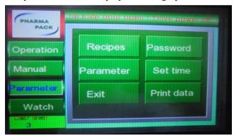
5.3.7 Press the "RECIPE" key from the above screen (It contains the different parameters used for setting of product ) and HMI will display:
