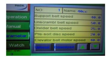
5.3.8 After "RECIPIE" press the "PARAMETER" key and HMI will display :
