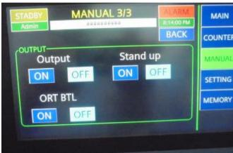
**NOTE:** "MANNUAL" has three pages displayed as 1/3, 2/3, 3/3. We can switch into different pages by pressing NEXT BACK. Press ON OFF key to start / stop the different parameters.
