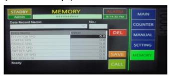
**NOTE:** "MEMORY" has saved data of previous run batches after pressing CALL we can load the previous message/values.
