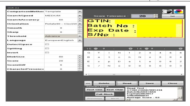
5.2.6 To set the threshold of OCR user has to uncheck click mark mentioned in dialogue box with yellow background. User must keep search accuracy in high mode for fast inspection. User can use smooth and sharp option for setting threshold. User must uncheck the splitting option from property. User must have to do check mark in DIVISION and SPECIAL CHARACTER in OCR property. User has to set score blob size and score difference. Now SAVE and TEST it. OCR AOI will show green in HMI.
