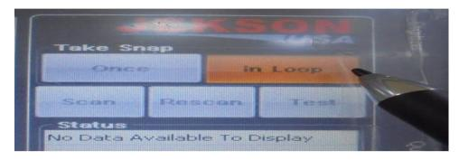
Pass one sticker label and printer will print the data and camera grabs an image of printed matter and Pharmacode. So user can see the image in IPC. If the image is dark or light user can change the camera setting from 'DIGITIZER' increase or decrease the shutter, brightness as per requirement display is mentioned below:-
