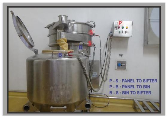
5.4.2.7. Fitted the sieve as per given in BMR for sifting and detached the clamps in sieve for neutralized the static charge generate during sifting.
